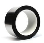
Carrier. PET/1.0 mil Adhesive/Thickness: Acrylic/1.1 mil Total Tape Thickness: 2.1 mil Adhesion to Steel: 29 oz/in Temperature Resistance: 250 ° F
